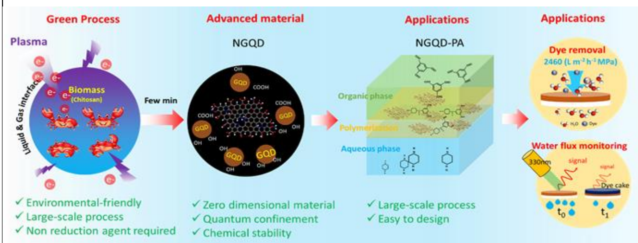
Figure 1. Schematic of microplasma-enabled biomass-derived NGQD/PA for multi-application.
